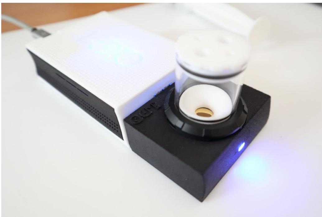
Fig. 11: Fully assembled electrochemical QCM system ready for combined measurements. The completed setup shows proper integration of all components: electrochemical module mounted on openQCM Q-1 platform
