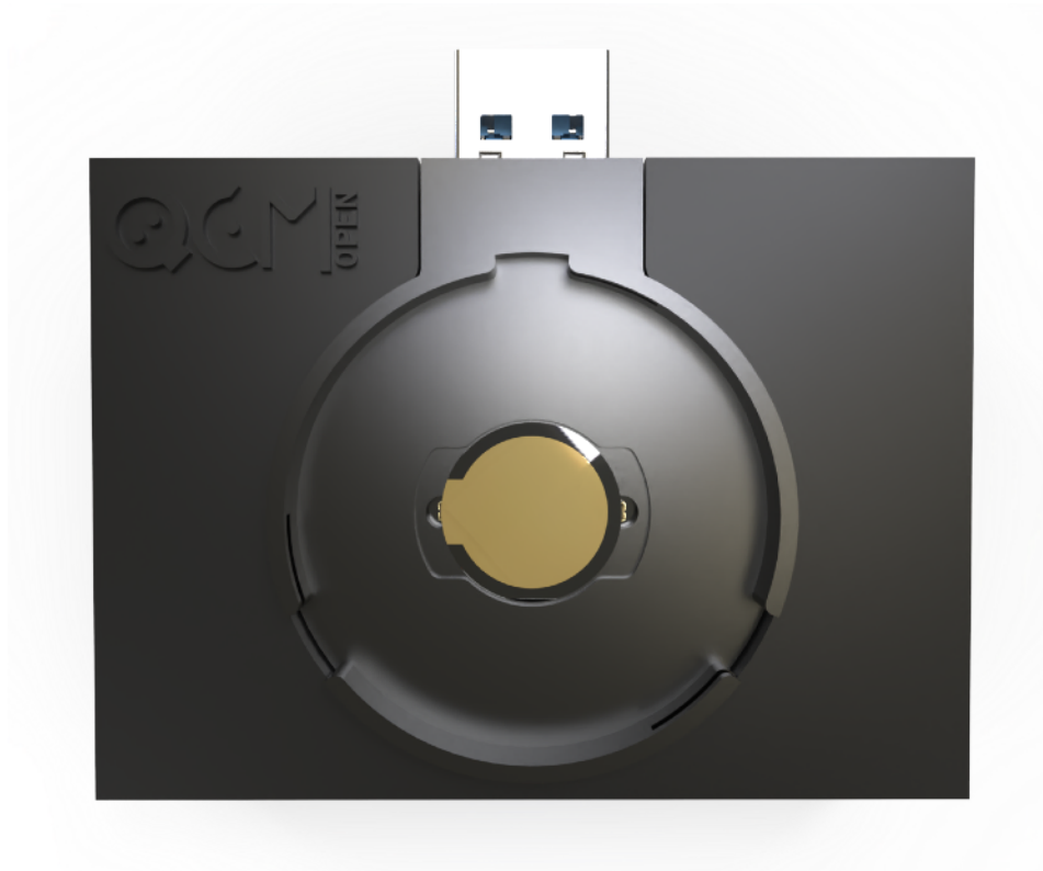
Fig. 4: orientation of the quartz sensor.
