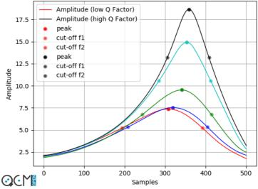
Q-factor is related to the dissipation D, which is a dimensionless parameter defined as the ratio between the energy loss and stored in each cycle:
