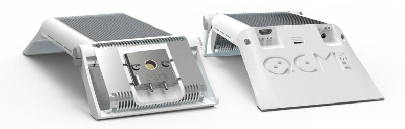
O penQCM NEXT design is the synthesis of all feedback received from the scientific community. We have come up with a characteristic bridge design, realised with the aim of maximising the thermal dissipation and electrical interferences of the electronics. The sensor module has been replaced with a custom heat sink, in which it is embedded a PTFE "slot", housing the fluidic module. The fluidic module is the real holder of the quartz sensors, made to be a multi-purpose accessory.
