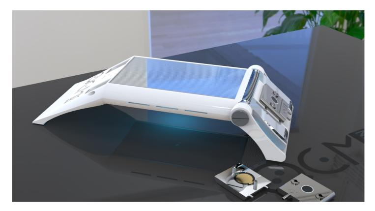
The Quartz Crystal Microbalance openQCM NEXT is a real-time analytical instrument based on a surface sensitive technology capable of monitoring phenomena at molecular scale. The NEXT is sensitive to mass and viscoelastic properties of molecular layers as they build up or change on the quartz sensor surface.
