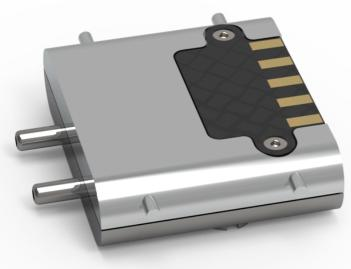
Just below the bottom quartz surface, a 10K thermistor monitors the internal temperature of the fluidic module. Electrical contact pads on its micro-PCB are produced by immersion gold technique. This process, drastically reduce the oxidation effects and consequently a degradation of S/N with the time.
